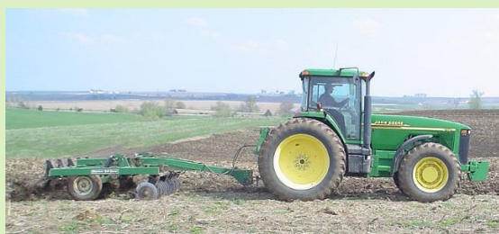
Pic. 1: Tractor with chisel plows, a good way to implement a reduced tillage with depth of around 15 cm; Pic. 2: Moldboard plows are tools used to achieve a more in-depth tillage (bad measure for soil conservation).
